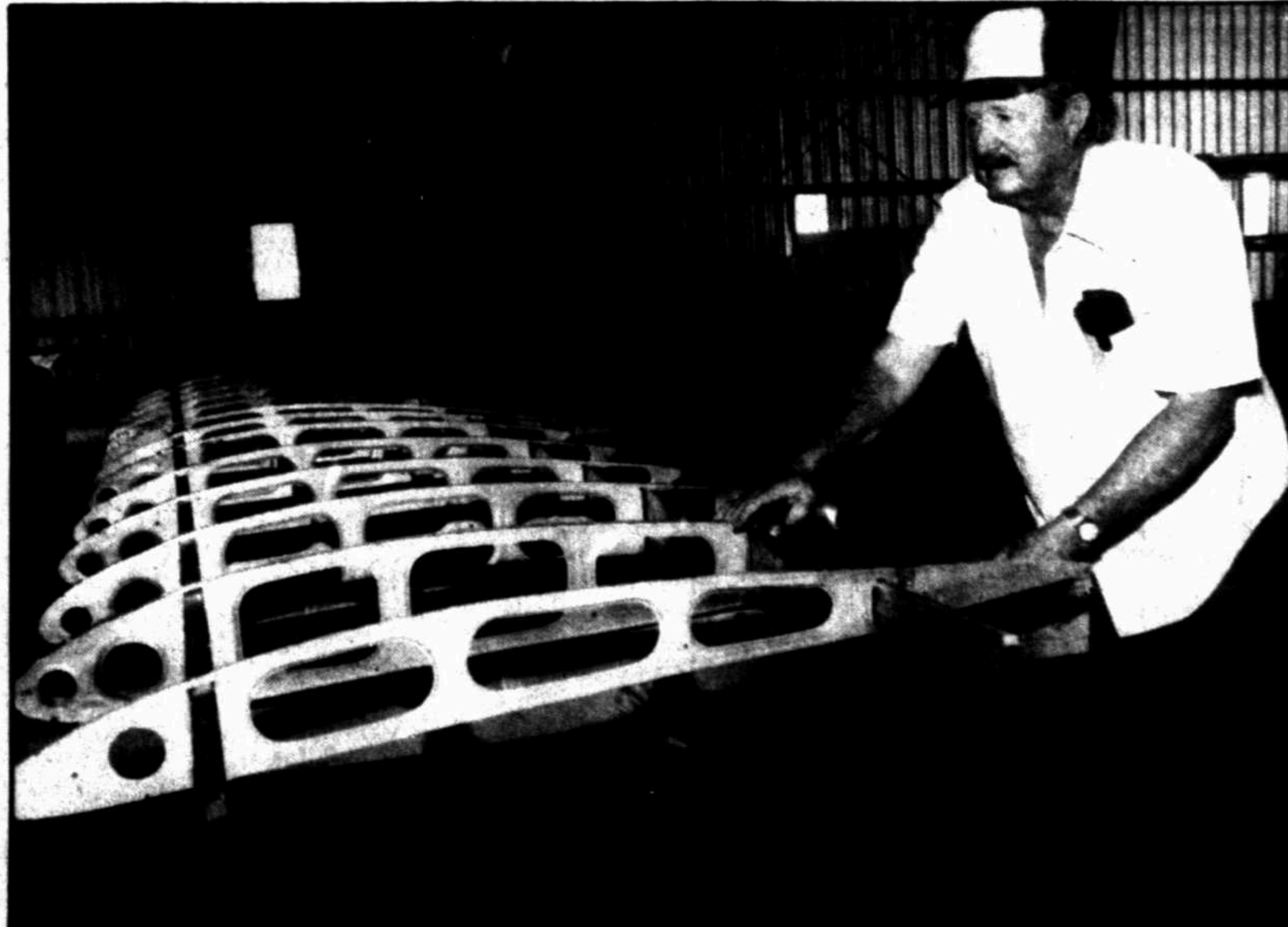
Each of these wing ribs is painstakingly set in place by craftsman Joe Whitaker.
