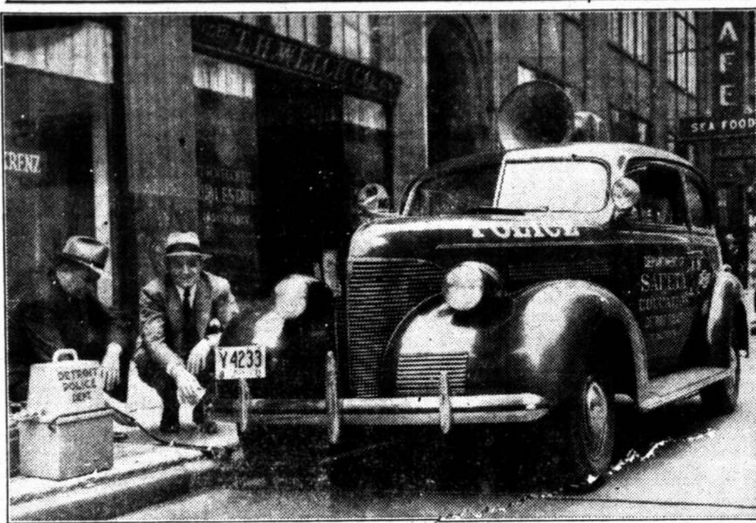
Detroit's recent decision to provide one-way streets to speed vehicle flow was made after extensive study of traffic. Modern science contributed to the survey with the "counter," an electrical recorder registering each car that passes it. A hose filled with compressed air extends half way across the street. As each car drives over it, an impulse is conveyed to the traffic counter, which automatically divides the impulses by two (in order to record each car as a unit) and prints a reading each half-hour. Show left discussing the equipment are M. W. Cochran, Detroit city traffic engineer (right), and John Wood, assistant chief engineer of Chevrolet.
