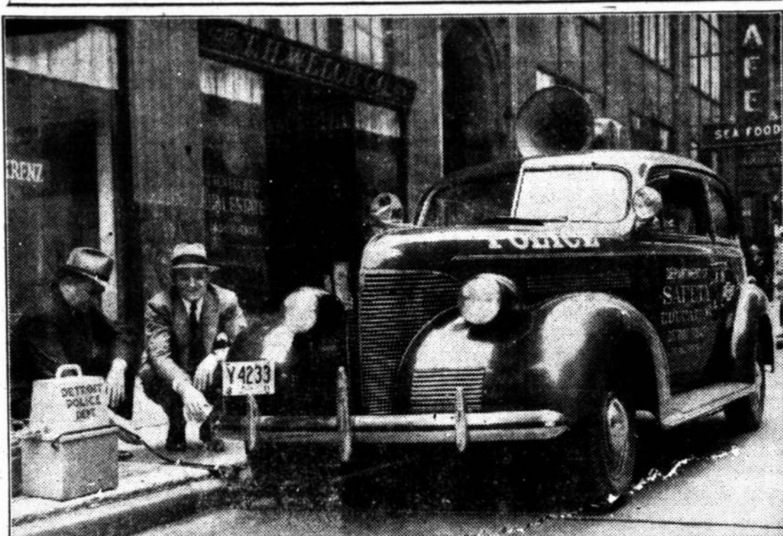
Detroit's recent decision to provide one-way streets to speed vehicle flow was made after extensive study of traffic. Modern science contributed to the survey with the use of an electrical recorder registering each car that passes it. A hose filled with compressed air extended half way across the street. As each car drives over it, an impulse is conveyed to the Trafficcounter, which automatically divides the impulses by two (in order to record each car as a unit) and prints a reading each half hour. Shown here discussing the equipment are M. W. Cochran, Detroit city traffic engineer (right), and John Wood, assistant chief engineer of Chevrolet.
