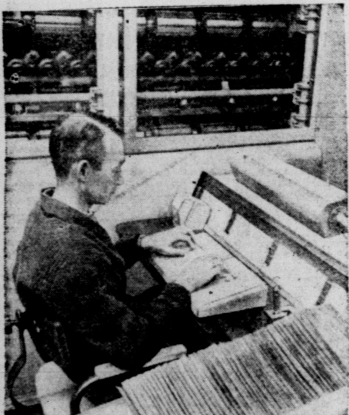
SET FOR SPEED —Clerk scans letter delivered by machine and prepares to punch proper key for sorting in nation's first automatic post office at Providence, R.I.
