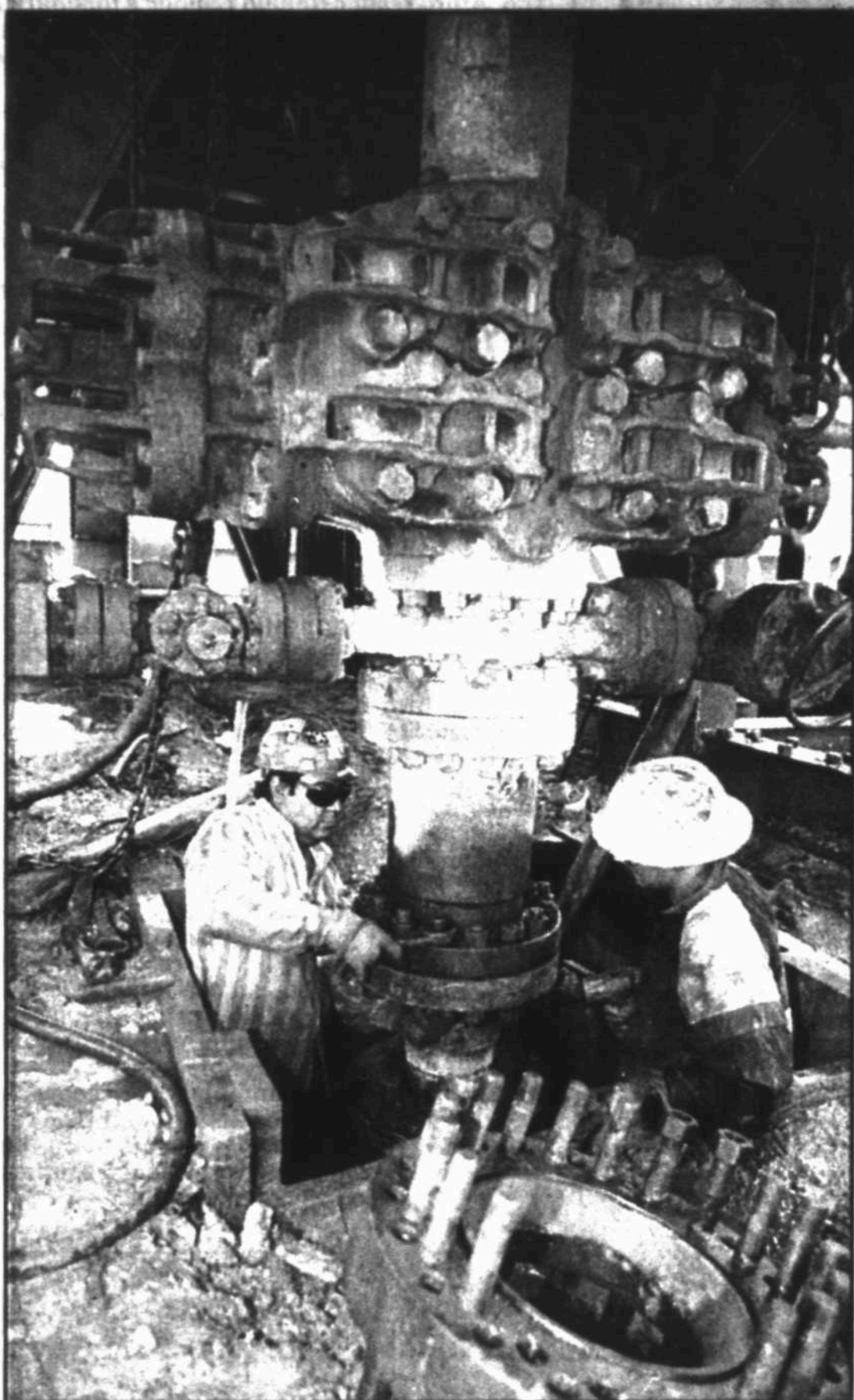
AP Photo Oscar Galindo, left, and Noe Marichalar, roughnecks with JSM Drilling Co., work together under the drilling rig floor, to nipple up a blowout preventer on a rig in the Spraberry Field south of Midland, Texas, in May 1997.
