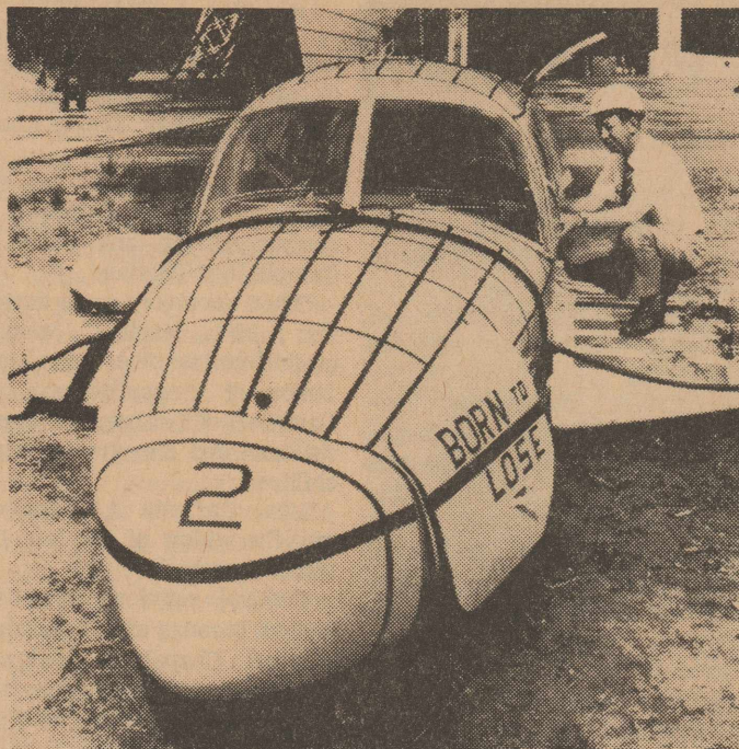
WHAT'S IN A NAME? This NASA test plane was built specifically to be crashed under controlled conditions to provide information on how to make airplane frames safer. The test site at Hampton, Virginia, has facilities to crash light aircraft at up to 60 miles an hour.
