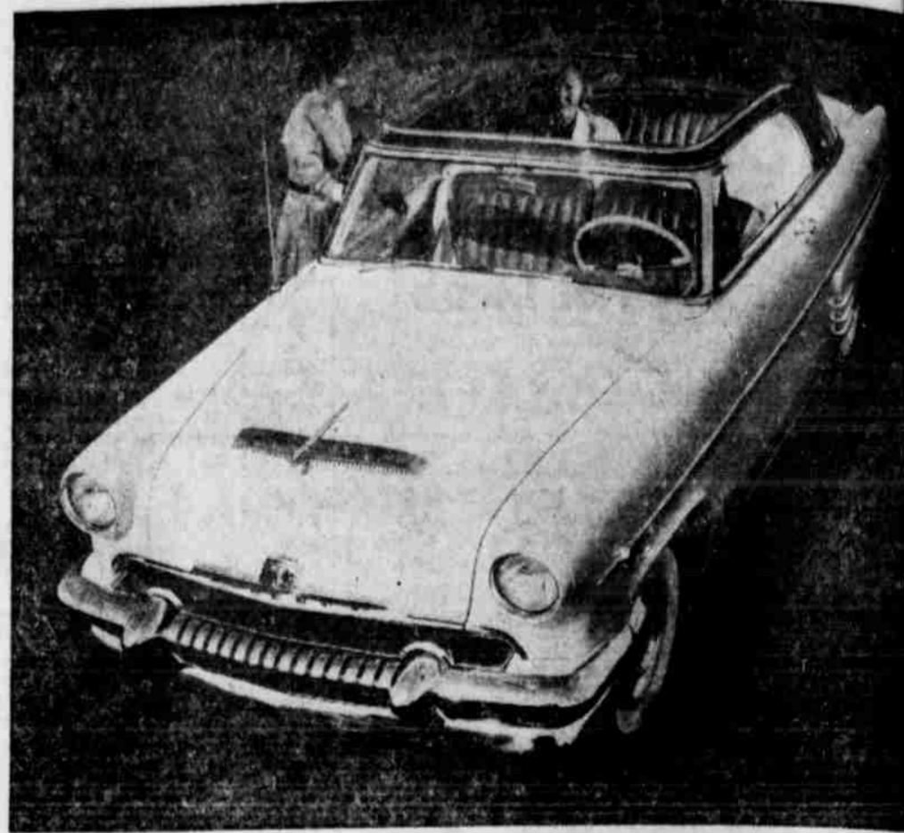
First new body style in the automobile industry since the hardtop! That's the Mercury Monterey "Sun Valley," a sports coupe with transparent plexiglas replacing over the front section of the roof. This quarter-inch thick plastic roof is tinted green to minimize light glare and is the first American production car of its type. Special trim combinations, and exclusive exterior color schemes characterize the "Sun Valley." Like all new 1954 Mercury models, it is powered by an entirely new overhead valve engine developing 161 horsepower.
