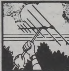
Antennas, ladders can contact danger
