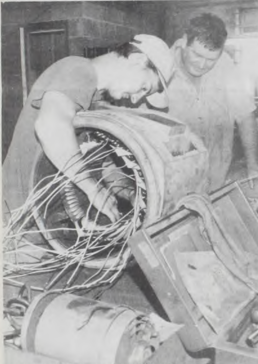
TODD SPARKMAN of Valley View rewinds a 50-horsepower oil field motor at United Electric Service on East Hwy. 82. Sparkman has a full-time summer job, working part-time at United for two years. Owner Harold Alexander oversees Sparkman's workmanship. United Electric has been at this location since 1972.
