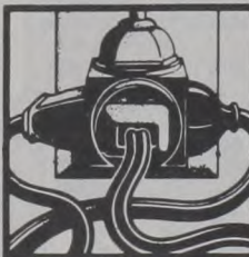
Don't overload outlets
