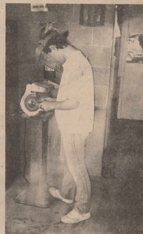
GRINDING MACHINE: Roby FFA members demonstrates grinder by grinding down a spur to desired shape.
