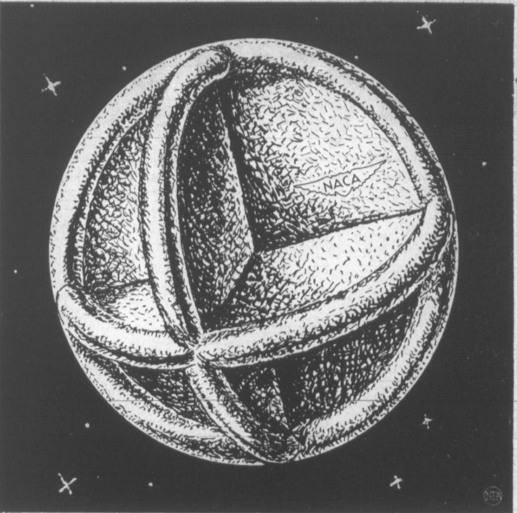
CORNERING SPACE —Artist's drawing above depicts the corner reflector sub-satellite developed by the National Advisory Committee for Aeronautics. The large but exceedingly lightweight earth satellite can be compactly folded for launching into orbit, and then pneumatically erected to shape by means of compressed air. It weighs only 8.7 pounds and when inflated it is 12 feet in diameter. Being in the shape of a corner reflector and covered with aluminum foil, the satellite will be the most efficient reflector of radar signals. Because of its large size, it would appear at twilight as bright as the North Star. If it were aimed so as to loop about the moon, its flight could be followed both going and returning. This would make it possible to verify calculations of the path that would be followed later by instrumental or manned space vehicles to be used for exploring space flight in the vicinity of the moon. It is constructed of Mylar plastic film 0.00025 inch thick that is covered with aluminum foil 0.0005 inch thick.
