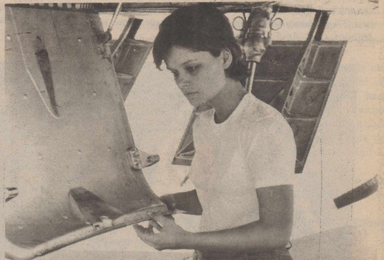
OPEN DOOR - Women on the flight-line is becoming an ever increasing sight. Here A1C Debbie Savage, an air frame repair specialist, inspects the seal on a T-38 gear door. (U.S. Air Force Photo by 2nd Lt. Ron Young)
