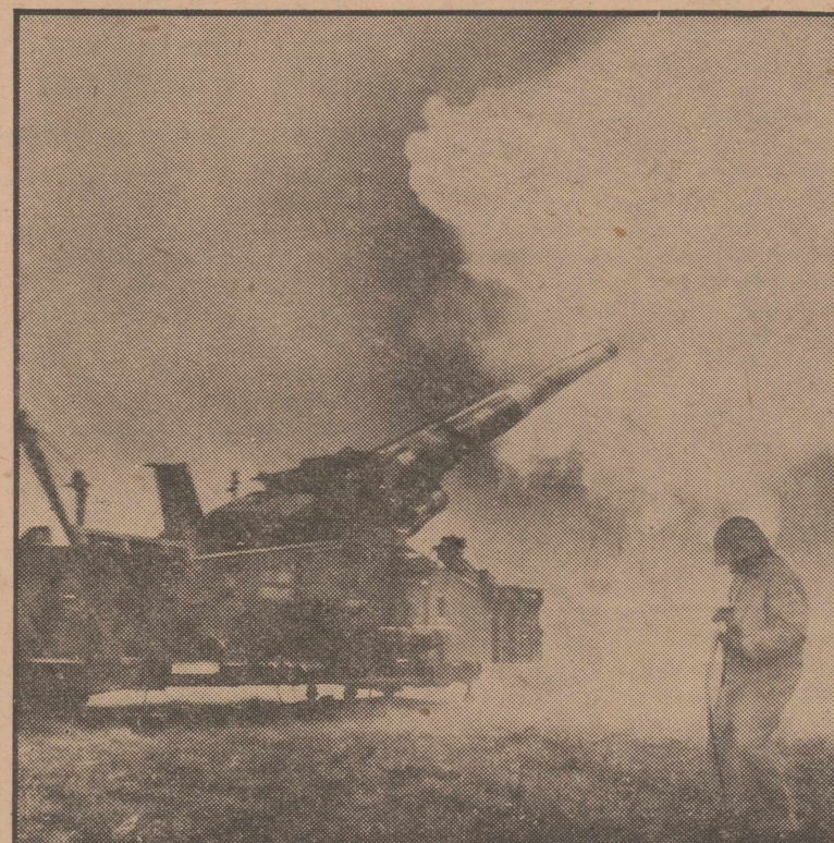
Big boom, and the 280-mm. shell screeches skyward for a test shot at Army Ordnance's Aberdeen, Md., proving ground. A civilian gunnery expert at the lanyard is seen at right. The projectile and powder charge are loaded into the gun's breech with hydraulic power hammer and may also be put in by hand.
