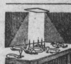
A center light on a table top reflects on a ceiling mirror to illuminate the whole table.
