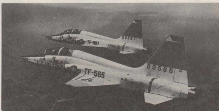
SUPERSONIC TALON —The supersonic T-38 Talon, newest training aircraft in the Air Force, provides basic pilot training for undergraduate pilot training students at Reese and the seven other UPT bases. With a top speed of about 850 mph, the T-38 is a trainer that makes it easier for a pilot right out of flying school to gain additional skills required to make transition to larger and faster-than-speed jets.
