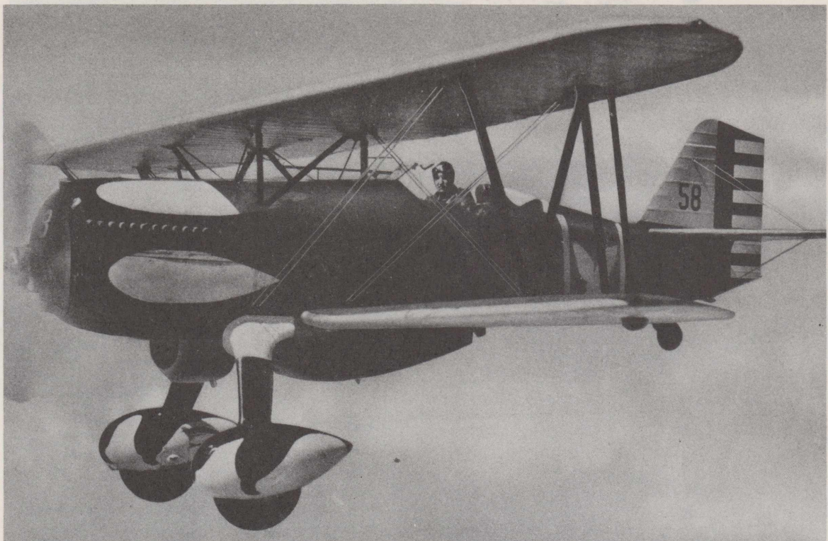
HISTORICAL AIRCRAFT —The Curtiss P-6E was the most famous of the Hawk series of pursuits. One of the most beautiful biplane fighters ever built for the Air Corps, it was highly maneuverable and armed with two synchronized machineguns. Powered by a 600-horsepower, liquid-cooled Curtis engine turning a three-bladed prop, this little fighter had a top speed of 197 miles per hour. A later model, the P-6F, was the first military aircraft to exceed 200 m.p.h. in level flight. (U. S. Air Force Photo)
