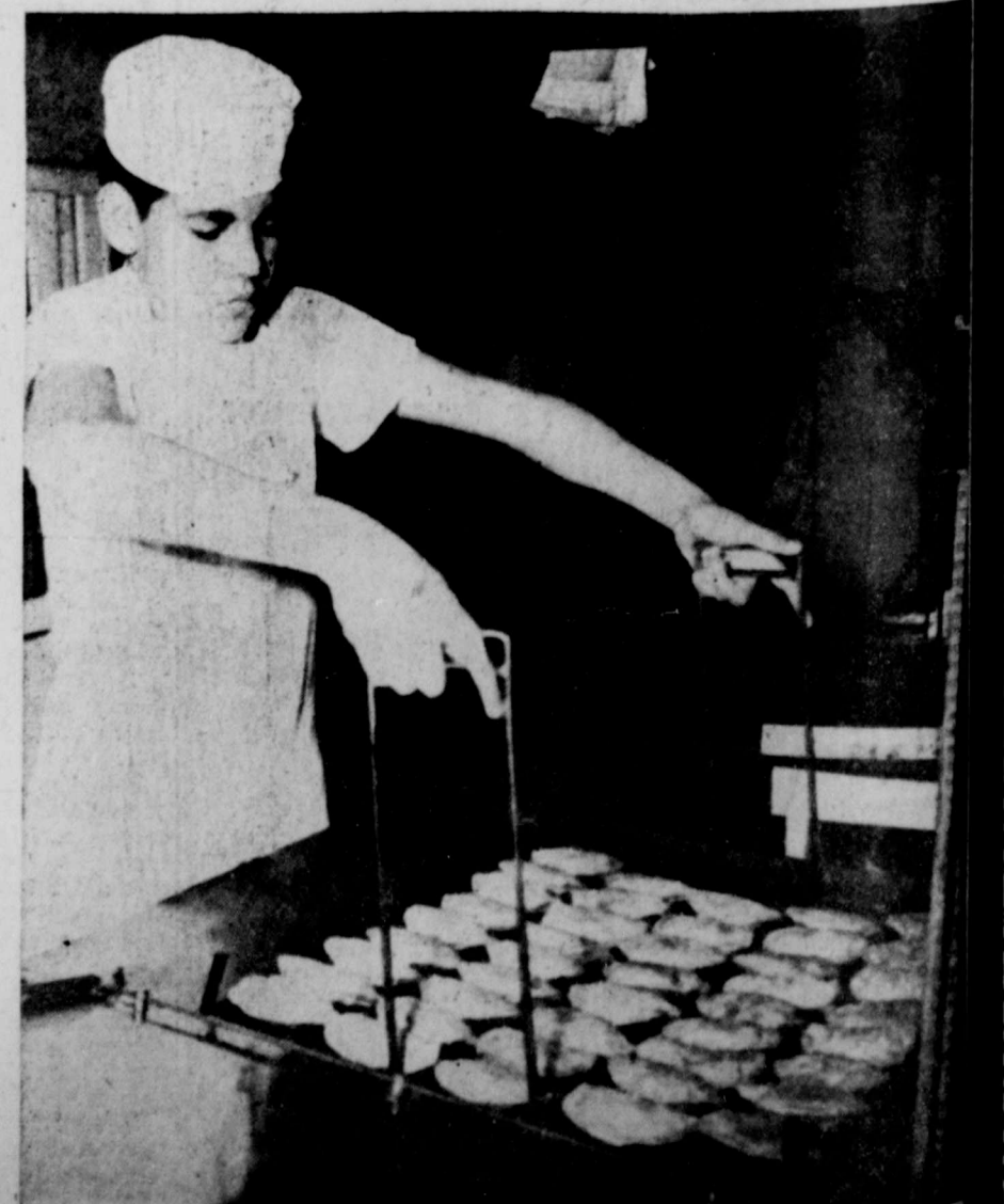
ZEKE DURAN lifts pies from the fry-o-lator. With this equipment Woodie Pie Company can turn out 45 fried pies every six minutes.
