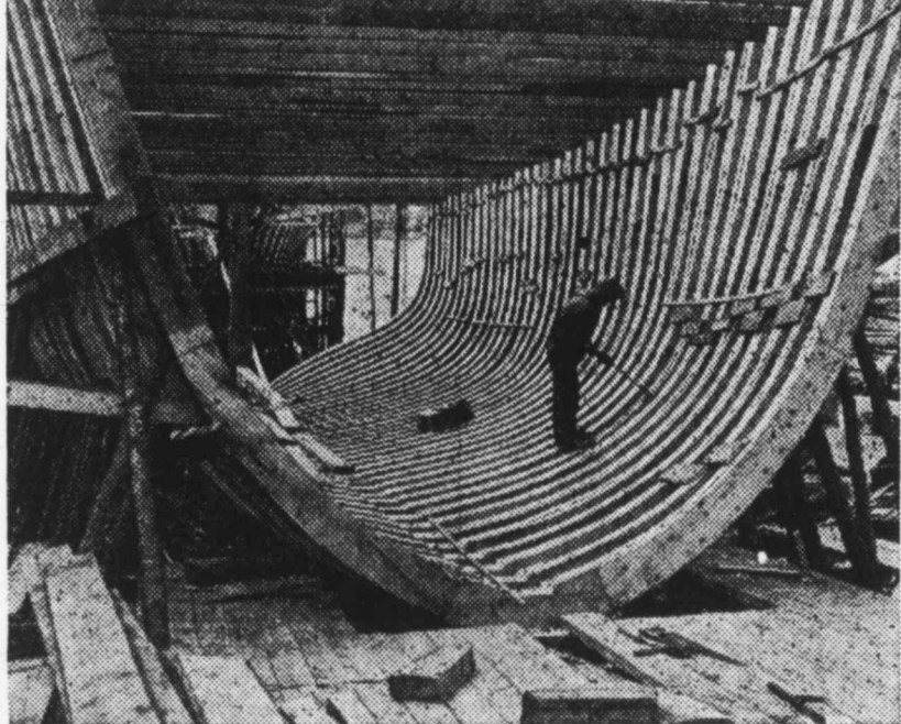
Old-timer Ray Rubshaw is working inside the framework of a hull under construction. He is dubbing or smoothing out and lining up the ribs for planking, using an adz.
