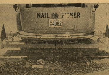
Electric magnets at the rear of the nail picker collect loose metal objects. The magnets are activated by a large generator in the bed of the truck and are strong enough to pock up manhole covers. Gathered in this pile of scrap metal are 2000 potential punctures.
