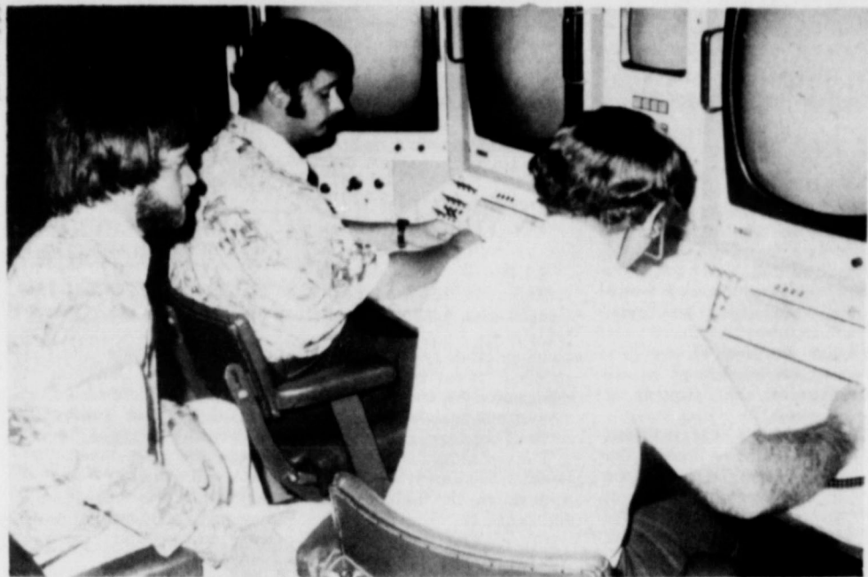
CONSOLE OPERATORS monitor the flights of four different simulator cockpits from a single station. The console operator will select variables such as visibility, wind, and navigation checkpoints for each simulator flight.
