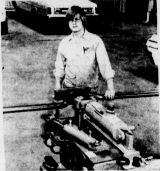
PRECISION BENDING—Gary Williams uses our new Huth pipe bender to make a customized 2-inch tailpipe for a Chevrolet pickup.
