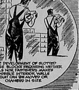
THE DEVELOPMENT OF SLOTTED GLASS BLOCKS REQUIRING NEITHER NAILS NOR FASTENERS MAKES POSSIBLE INTERIOR WALLS THAT CAN BE MOVED OR CHANGED IN SIZE.
