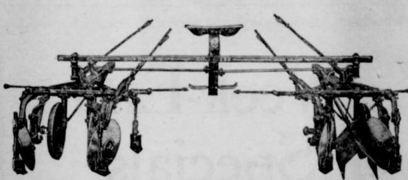
There are four levers on the Rock Island No. 126 Cultivator, all located conveniently for the operator, there being one shovel adjusting lever and one raising lever on each side. Double plunger construction on the shovel levers gives fine depth adjustments-twice as fine as on other cultivators
