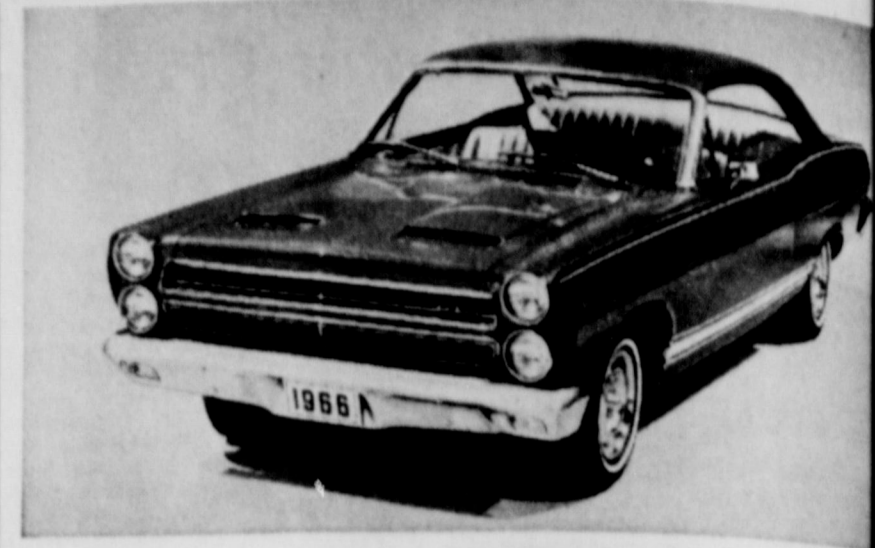
Completely restyled for 1966, Comet features a new larger body, a wider choice of engines. Overall length has been increased 1 1/2 inches and wheelbase is two inches greater at 116 inches. Two Mercury engines are added to the power offerings. Sportiest of the new Comets is the model (above) which offers a high performance 335-horsepower V-8 engine with fiberglass hood with simulated air scoops. The 1966 Comet goes on sale Oct. 1.
