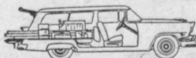
With "Stowaway" seat hidden in floor, you have almost 8 feet of cargo room from front seat to end of tailgate.
