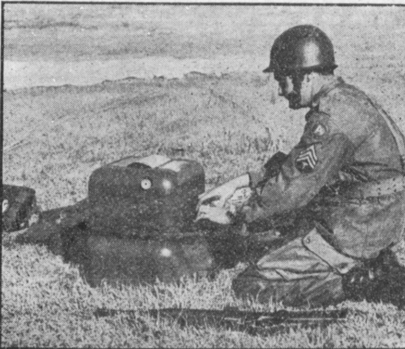
Cpl. William A. Allen of Corpus Christi, Tex., sets to work on a new portable teletypewriter after jumping from a C-82 plane with it (and a parachute). The airborne machine, developed especially for use by Army Signal Corps paratroopers, was tested in demonstrations like this at Fort Bragg, N. C.
