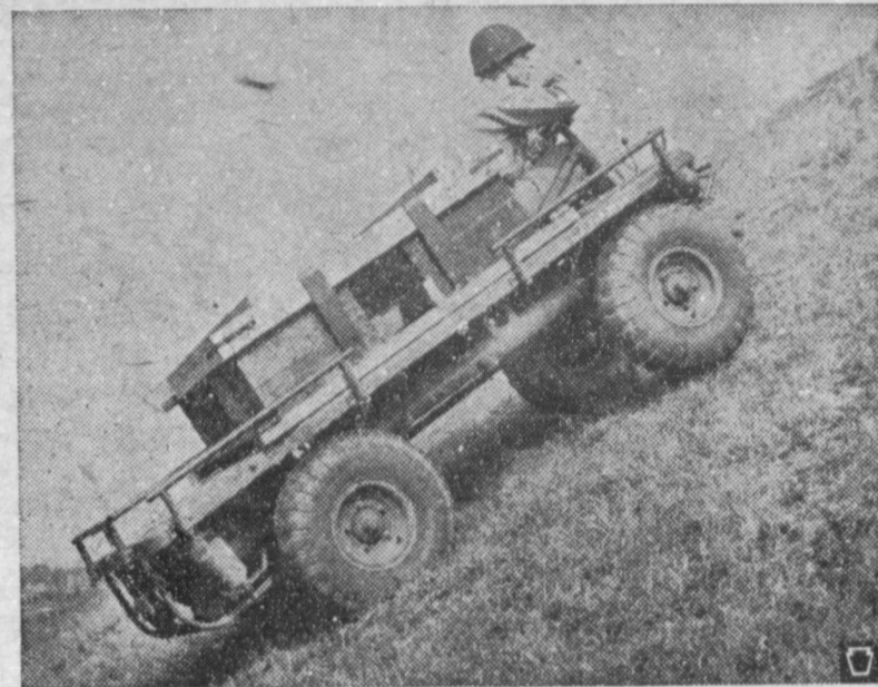
The "Mechanical Mule," modern gasoline burning version of the traditional old Army hay-burner, is going into service to "take the load off the foot soldier's back." Equipped with 4-wheel drive, it can carry more than its own weight up hills, across streams and over the roughest terrain. It also can be transported by helicopter and dropped by parachute for airborne troop operations. Designed by Willys Motors, Inc., under Army Ordnance supervision, the Mechanical Mule will go into production at the Willys Jeep plant in Toledo with first deliveries scheduled to be made to the famed "Screaming Eagles" 101st Airborne Division.
