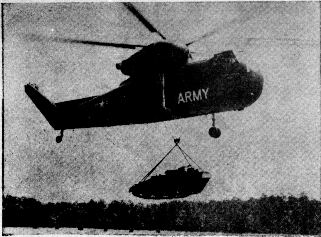
ARMY'S BIGGEST —The twin-engine, all-metal H-37 "Mojave" helicopter was designed to carry 36 combat soldiers, evacuate 24 litter patients, or carry cargo. As the Army's largest 'chopper, it's a "going concern" in Transportation Corps helicopter companies available to support units of the pentomic Army. Here it easily carries a 15,000-lb. "Scorpion," a full-tracked, self-propelled armored vehicle which mounts a high-velocity 90mm anti-tank gun.
