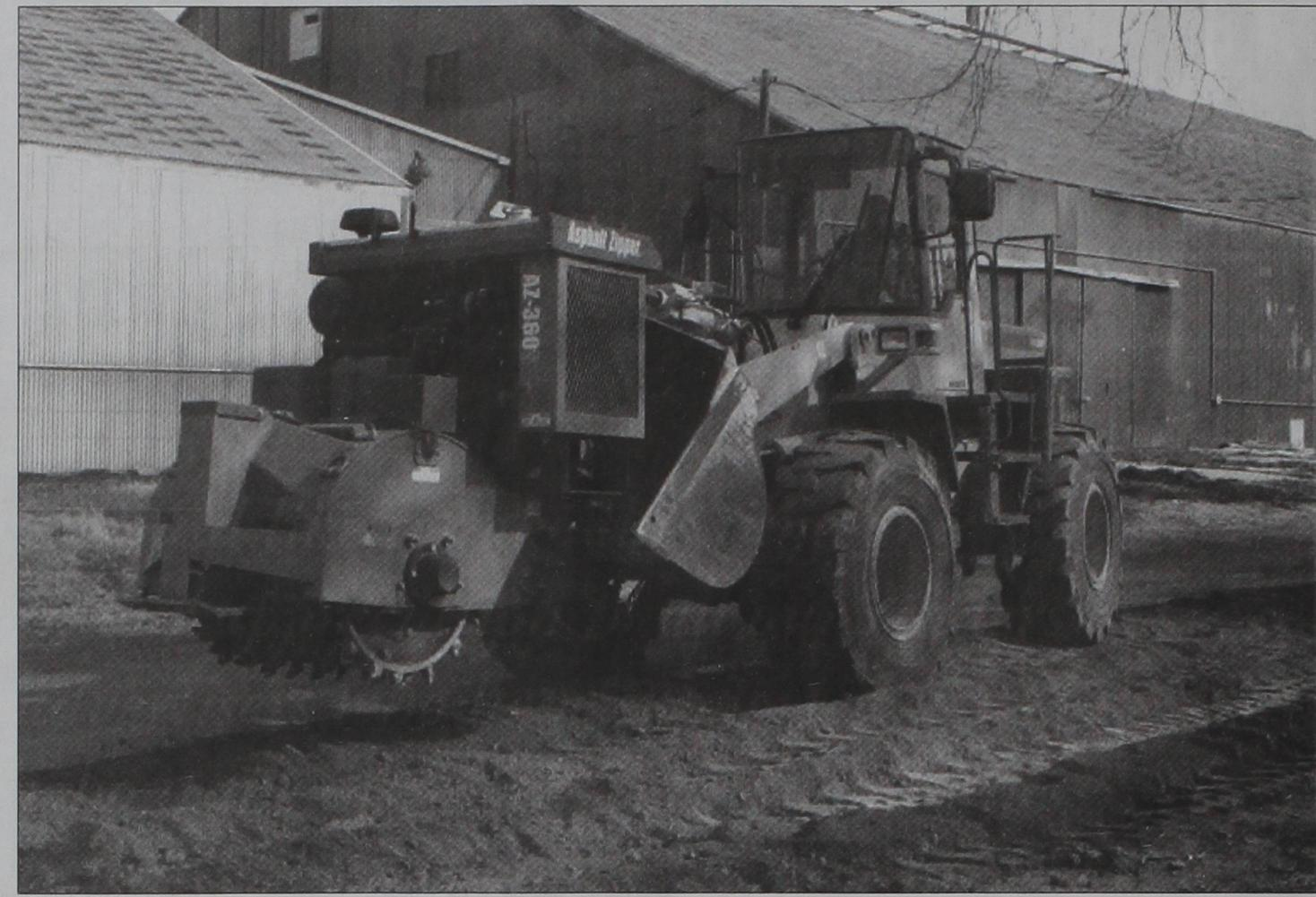
The City of Clarendon made short work of a bunch of potholes when it began working with its new Asphalt Zipper last Wednesday. The device attaches to a front-end loader and makes a clean cut as it grinds up pavement and potholes. Dry cement is then mixed into the millings, which is later wetted and bladed to creat a smooth new base. The city hopes to use the Zipper repair badly deteriorated
