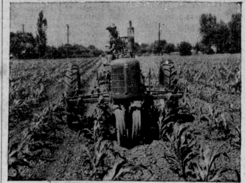
For planting and cultivating two, four or six rows, the Farmall C tractor is an ideal unit. This tractor, built by International Harvester, is designed for diversified farms of up to 120 acres; for large-scale vegetable farms, and as "second tractor" power for large-acreage farms. Shown here with two-row cultivator, doing a clean, fast job in corn.
