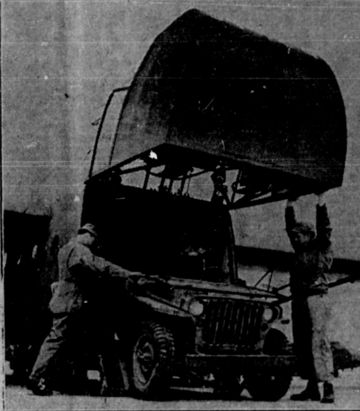
Released by U. S. War Department Bureau of Public Relations FLYING FREIGHT CAR —In carrying a jeep on a glider, the entire pilot's compartment lifts on hinges. The same procedure is followed in loading artillery.
