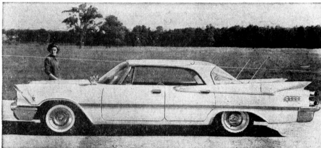
The tail fins of 1959 Dodge cars, like this Custom Royal four-door Lancer, have softer, more flaring lines. A new high-contour roof provides more headroom and allows easier entry and exit. New engines and advanced torsion-ride suspension provide greater gas and tire economies.
