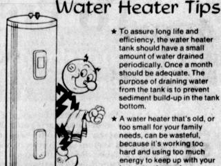
★ To assure long life and efficiency, the water heater tank should have a small amount of water drained periodically. Once a month should be adequate. The purpose of draining water from the tank is to prevent sediment build-up in the tank
