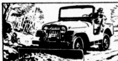
Hydraulic lift. With hydraulic lift, the 4-wheel drive 'Jeep' operates graders, scrapers, post hole diggers and most 3-point hitch implements.
