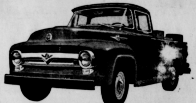
NEW FORD F-100 8-FT. 1/2-TON PICKUP. GVW 5,000 lbs. Choice of 133-h.p. Six or 167-h.p. V-8.
