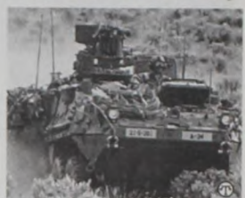
Traveling at speeds of 62 mph a new combat vehicle called the Stryker is changing the way the Army will fight.
