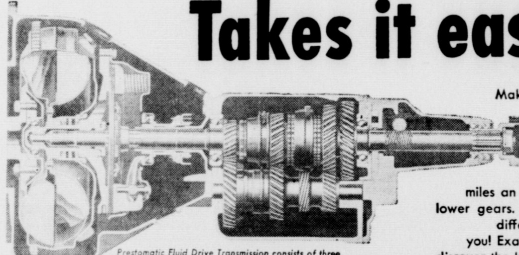
Prestomatic Fluid Drive Transmission consists of three compact units — Fluid Drive, the Safety Clutch and Prestomatic Transmission. Each unit is designed with a minimum of moving parts, and each unit is ruggedly built to give trouble-free service for the lifetime of the car.
