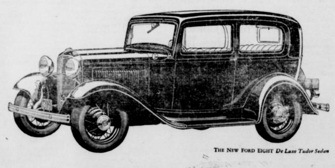
Eight-cylinder, 90-degree V-type, 65-horse-power Engine \* Vibrationless Roomy, Beautiful Bodies \* Low Center of Gravity \* Silent Second Gear Synchronized Silent Gear Shift \* Seventy-Live Miles per Hour \* Comfortable
