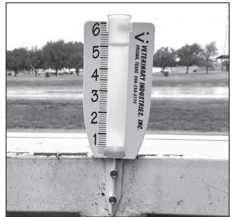
The Friona Star rain gauge shows the first five inches of rain that fell on November 2nd. Notice that the bottom .2 portion of the gauge is discolored because most of our rains this past year were that amount.
