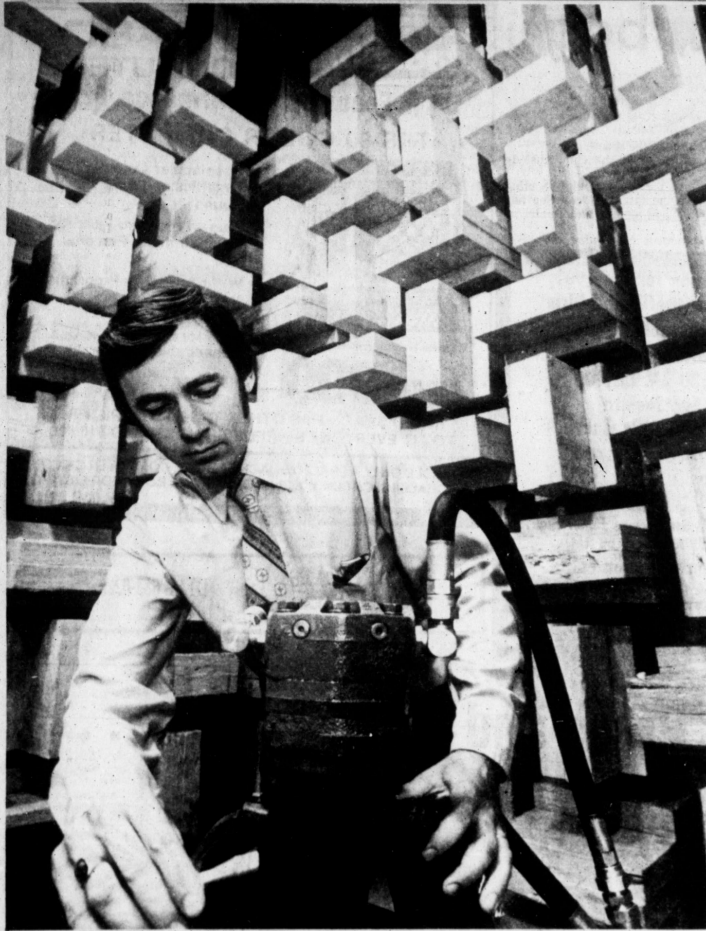
DuWayne Bohlman, a project test engineer for J.I. Case Company, tests the noise level of a hydraulic pump in a futuristic-looking "quiet room" at the company's Drott Division plant in
