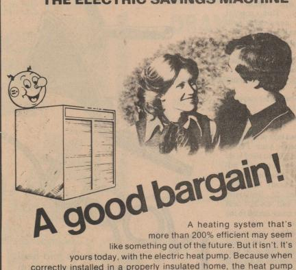
correctly installed in a properly insulated home, the heat pump produces two units of heat for each single unit of electricity it uses. The heat pump operates by using the future's most abundant energy source, solar energy. It transfers heat that's always present in sun-warmed outside air into your home during the winter. And reverses the process, pumping heat outdoors during the summer.
