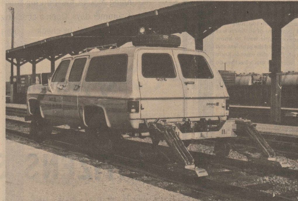
SANTA FE RAILWAY is one of the first railroads to turn exclusively to ultrasonic testing for internal rail flaws. Pictured above is one of the railroad's five ultrasonic rail detector cars now in service on the Santa Fe system. (Photo courtesy Santa Fe Railway)
