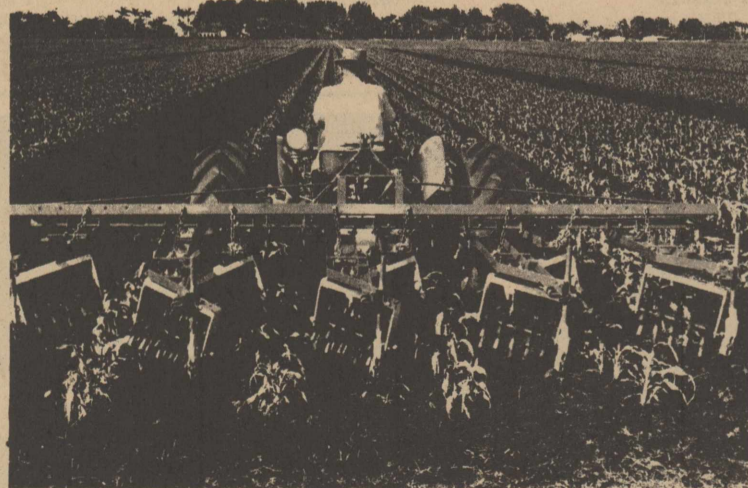
Here, the Rolling Cultivator is set to throw dirt toward the corn. The higher the angle, the higher the bed. Adjustments are simple, take only minutes to make.
