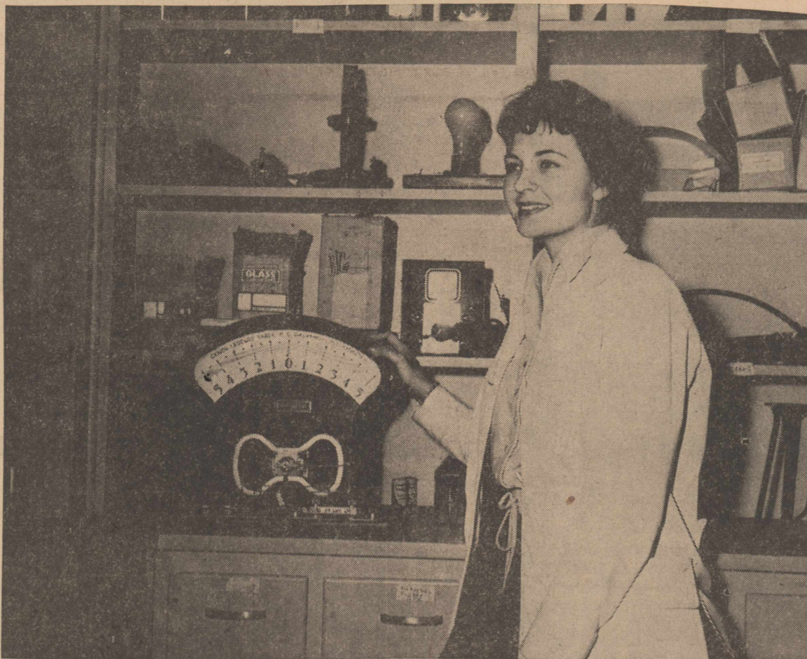
Ronda Robertson is shown with an additional piece of equipment recently acquired by Olton High School science department. It is a galvanometer donated by Doug Sopher, who farms northeast of Olton. The device is used to show electric currents and voltages in demonstrations and experiments before an entire class. (STAFF PHOTO)
