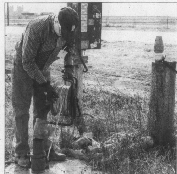
Taking measurements... HPWD Field Staff Supervisor Keith Whitworth uses an E-Line to make a water level measurement in an observation well.
