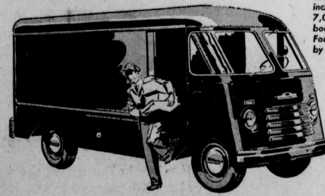
LIGHT-DUTY DE LUXE PANEL* Model 3105—116-inch wheelbase, Maximum G.V.W. 4,600 lb. Also available in Medium-Duty model 3805—137-inch wheelbase, Maximum G.V.W. 6,700 lb.
