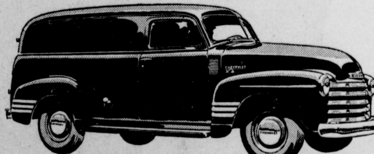
LIGHT-DUTY DE LUXE PANEL* Model 3105—116-inch wheelbase, Maximum G.V.W. 4,600 lb. Also available in Medium-Duty model 3805—137-inch wheelbase, Maximum G.V.W. 6,700 lb.
