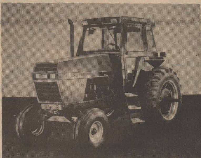
This is the new Case IH farm machinery. Note the combination of the logo for the new equipment. This is the Model 2096 Agricultural tractor rated at 115 PTO horsepower.
