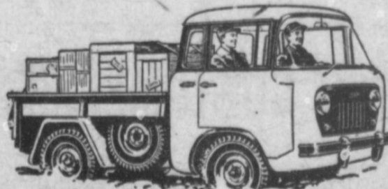
The New Forward Control 'Jeep' FC-150... puts a 74" pickup box on a wheelbase only 81" long.
