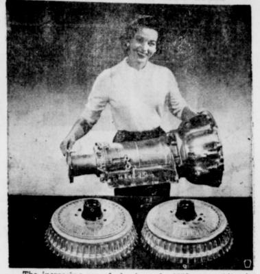
The increasing use of aluminum in 1958 automobiles is demonstrated by this pretty model holding a 26-pound housing for Buick's new flight pitch Dynaflow transmission. The transmission case and the air-cooled brake drums make up 44 of the 95 pounds of aluminum Buick will use in some of its 1958 models. About 180 pounds of weight is saved by the use of aluminum instead of the traditional cast iron.
