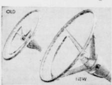
1. NEW IMPACT-ABSORBING STEERING WHEEL with deeply recessed hub and 3-spoke conical design bends under impact or pressure. The driver is better protected in case of accident.
