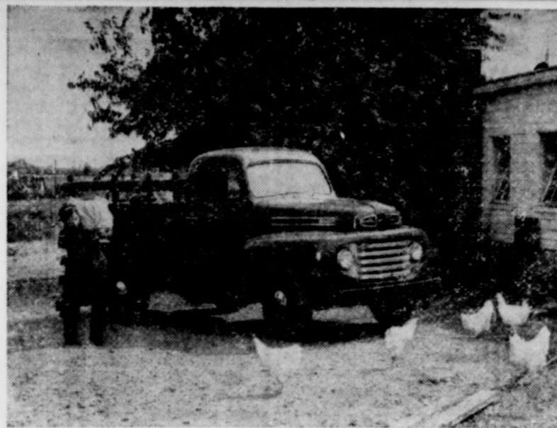
SERIES F3 1950 model Ford truck with stake body. Maximum gross vehicle weight rating is 6,890 pounds. An eight-foot express body also is provided. One of 175 new 1950 model Ford trucks.
