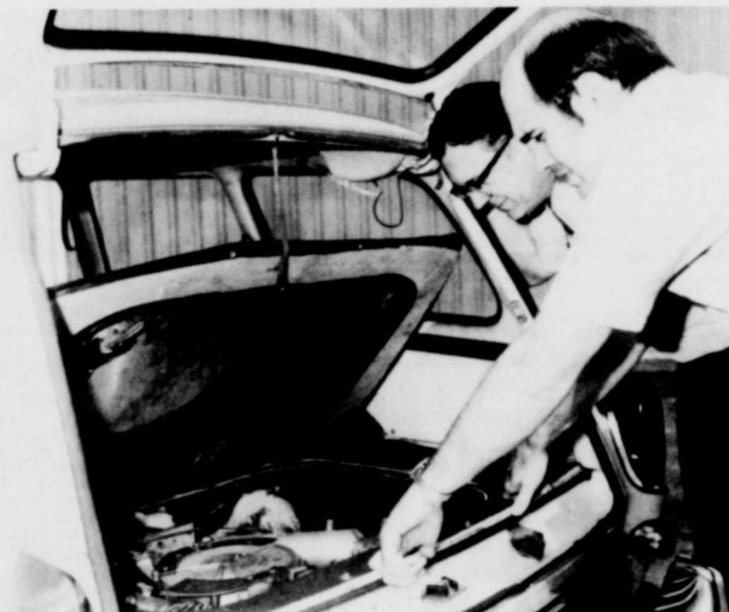
STEAM ENGINE--Jay W. Carter and Jay W. Carter, Jr. check the steam engine they installed in a 1964 Volkswagen. The engine was the very first in the nation to pass the rigid 1976 emission control standards set by
